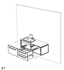
Apply a white silicone sealant between the back side of the tabletop and the wall. Connect the water supply and drainage. Vipp recommends you to use certified installer for both jobs.
